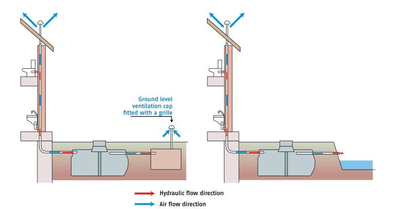
If the drainage channelling contains an anti-return flap, the diagram on the left applies.
